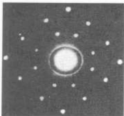
FIGURE 4.7 Diffraction of neutrons by a sodium chloride crystal.
