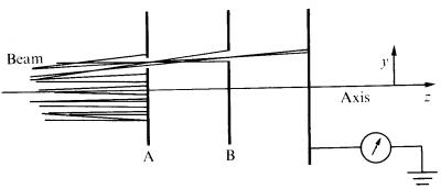
The combination of two slits give position and divergence → direct emittance measurement. Applicable for space charge dominated beams (if slits are small enough).
