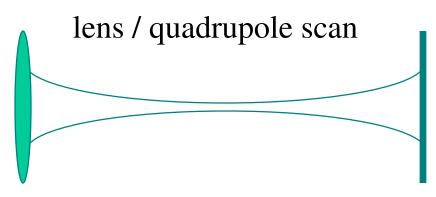
We'll see later that envelope equation in drift is  $\sigma'' \approx \frac{1}{2I_0} \frac{1}{\gamma^3 \sigma} + \frac{\varepsilon^2}{\sigma^3}$
