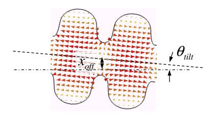
• One would prefer on-crest running in the injector (and elsewhere!) from tolerances' point of view
