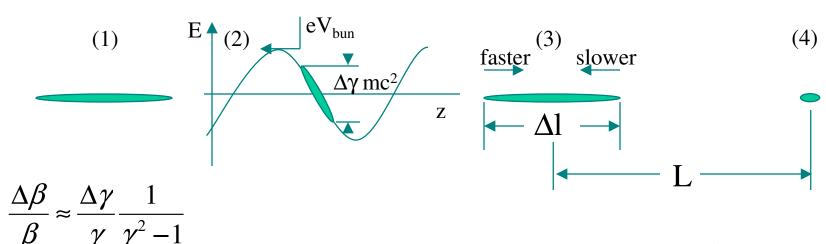
$$L = c\beta \frac{\Delta l}{c\Delta\beta} = \frac{\Delta l}{(\Delta\gamma/\gamma)} (\gamma^2 - 1) = \frac{\lambda_{RF}}{2\pi} \frac{E}{eV_{bun}} \left( \frac{E^2}{(mc^2)^2} - 1 \right)$$
