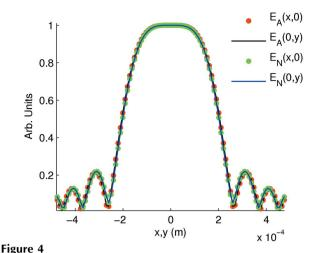
Undulator radiation electric field amplitude computed numerically  $(E_N)$  and analytically  $(E_A)$ . Slices are shown at x = 0 and y = 0 to demonstrate rotational symmetry.
