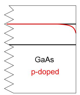
Charge accumulates in the lowered potential at the surface and builds a strong barrier for the emission of electrons.
