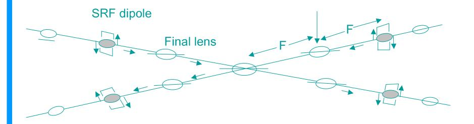
Parasitic collisions are avoided without loss of luminosity
