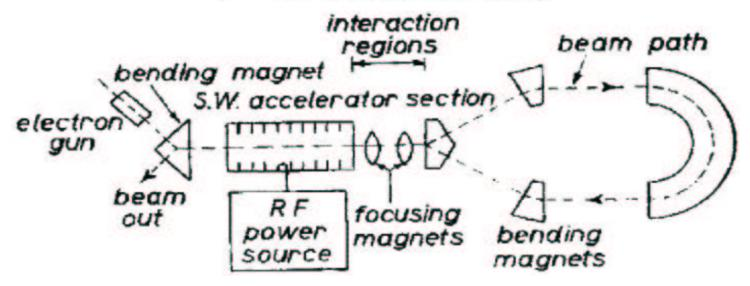
Energy recovery needs continuously fields in the RF structure
