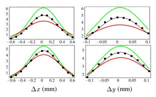
Figure 2: The luminosity scan at H1 for the 72° test optics before the upgrade. Left: horizontal. Right: vertical. The curves show the luminosity data (dots) and a Gaussian fit (black) together with the luminosity (green, upper curve) expected by method a) and the luminosity (red, lower curve) expected by method (b) from the area under the fit. Top: before, Bottom: after taking into account the beam—beam kick and the beam—beam focusing.
