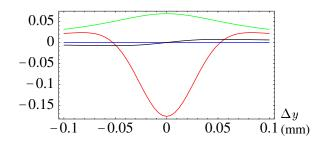
Figure 1: Perturbations due to the beam–beam effect during a luminosity scan in HERA's phase 2. In each figure the central curves describe the beam–beam displacements  $\delta x$  (blue) and  $\delta y$  (black) in mm. The lowest (red) and the highest (green) curves describe the relative change  $\delta\beta_y^e/\beta_y^e$  and  $\delta\beta_x^e/\beta_x^e$  of the beta functions respectively.
