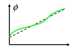
$$\begin{pmatrix} x \\ a \end{pmatrix} = \sqrt{2J} \begin{pmatrix} \sqrt{\beta} & 0 \\ -\frac{\alpha}{\sqrt{\beta}} & \frac{1}{\sqrt{\beta}} \end{pmatrix} \begin{pmatrix} \sin(\psi - \mu \frac{s}{L} + \varphi) \\ \cos(\psi - \mu \frac{s}{L} + \varphi) \end{pmatrix} \Rightarrow J' = 0$$
