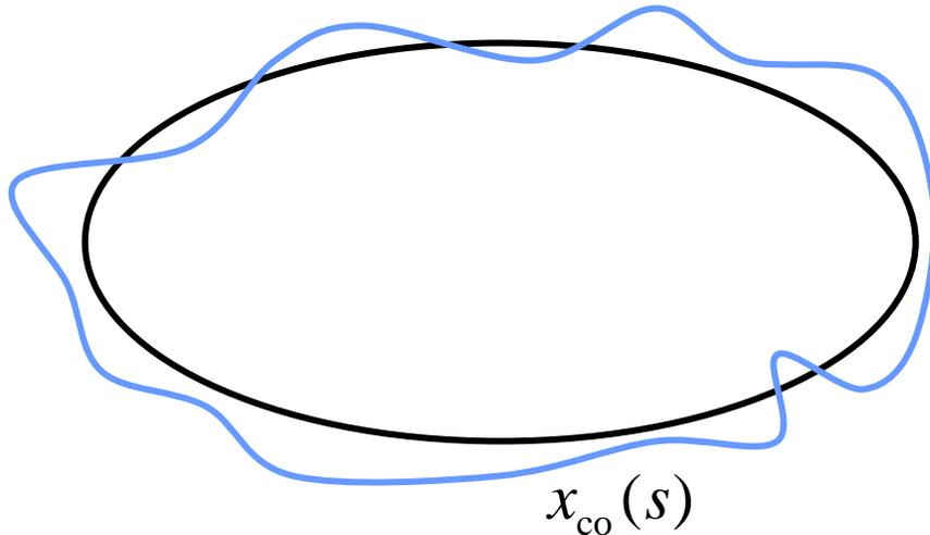
Particles oscillate around this periodic orbit, not around the design orbit.
