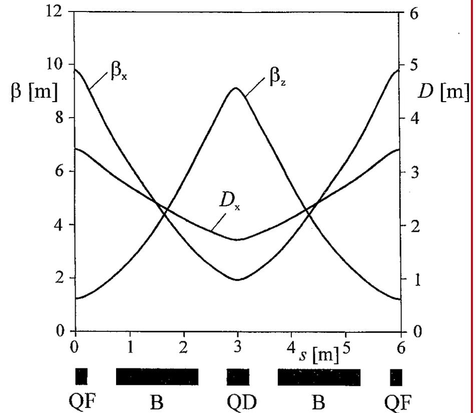
$$L_{FoDo} \approx 6\text{m}, \quad \varphi \approx 22.5^\circ, \quad \mu_{FoDo} \approx \frac{\pi}{2}$$
