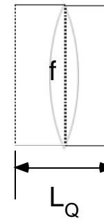
The transport matrix for a physical lens of length  $L_Q$ , in the thin-lens approximation, is the matrix product:
