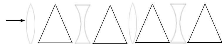
Linear particle transport through each element corresponds to multiplication by the appropriate  $\mathbf{M}$  matrix. The alternating gradient provides strong focusing in both planes.
