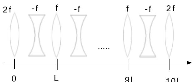
Symmetric FODO lattice, no bends. 10 cells  $L=1$  m. Lens focal length  $f$ . Let  $\mathbf{M}_c(f, s, 0)$  = transfer matrix from 0 to  $s$  for symmetric FODO cell of focal length  $f$ .
