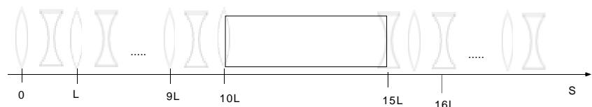
10 cell Symmetric FODO lattice focal length  $f$ , 5 m bend with  $\phi=0.1$ , 10 cell symmetric FODO lattice, focal length  $-f$ .  $L=1$  m.
