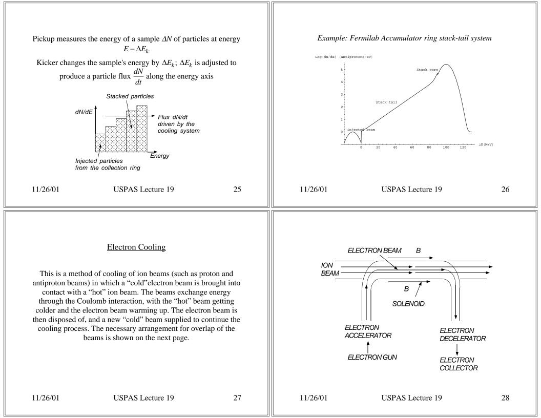
The mechanism for energy exchange between the electrons and the ions is the same as the one responsible for ionization energy loss. The strength of this interaction is maximum when the ions and the electrons are at rest with respect to each other: for two beams, this requires that the beams have equal velocities:
