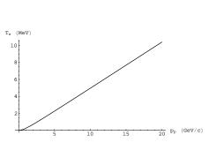
Substantial electron energies (MeV) and currents (amps) are required for high energy electron cooling, which is why it is important to recover essentially all of the electron beam energy in the collector.
