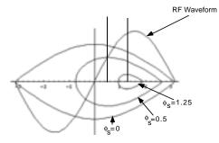
The *bucket area*, the area within the separatrix (in  $\Delta E$ ,  $\Delta t$  phase space), can be found by integrating over the bucket; the result is
