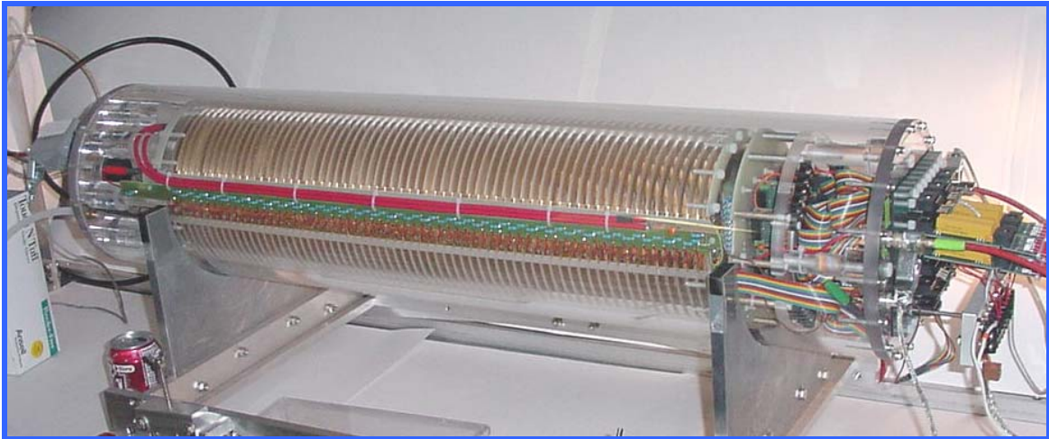
Figure 2: Time Projection Chamber at Cornell University. The drift cage has an inner diameter of 14.6 cm and length of 64 cm.
