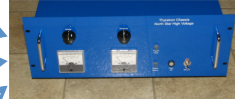
Thyatron Chassis with Driver, Heater and Reservoir Power
