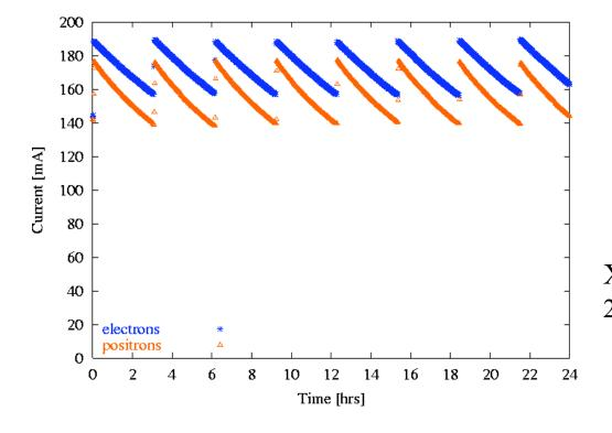
200 mA - 30 bunches electrons 180 mA - 22 bunches positrons  $\tau \sim 12$  hours Periodic top off ~ 3hours (Top off in 3 minutes)  $\epsilon_h \sim 140$  nm  $\epsilon_v \sim 1-2$  nm X-ray beam position stability < 30 µm. 23.5 hours beam/day
