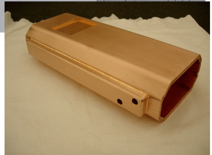
Machining & Welding Test Piece (LBNL)
