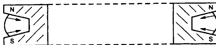
Figure 3.3. Cross section of weak focusing circular accelerator.
