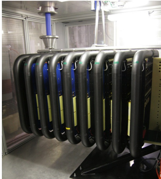
Figure 2.5. Prototype 120 kV Marx modulator.
