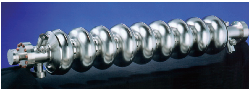
Figure 2.2. A 1.3 GHz superconducting nine-cell niobium cavity.
