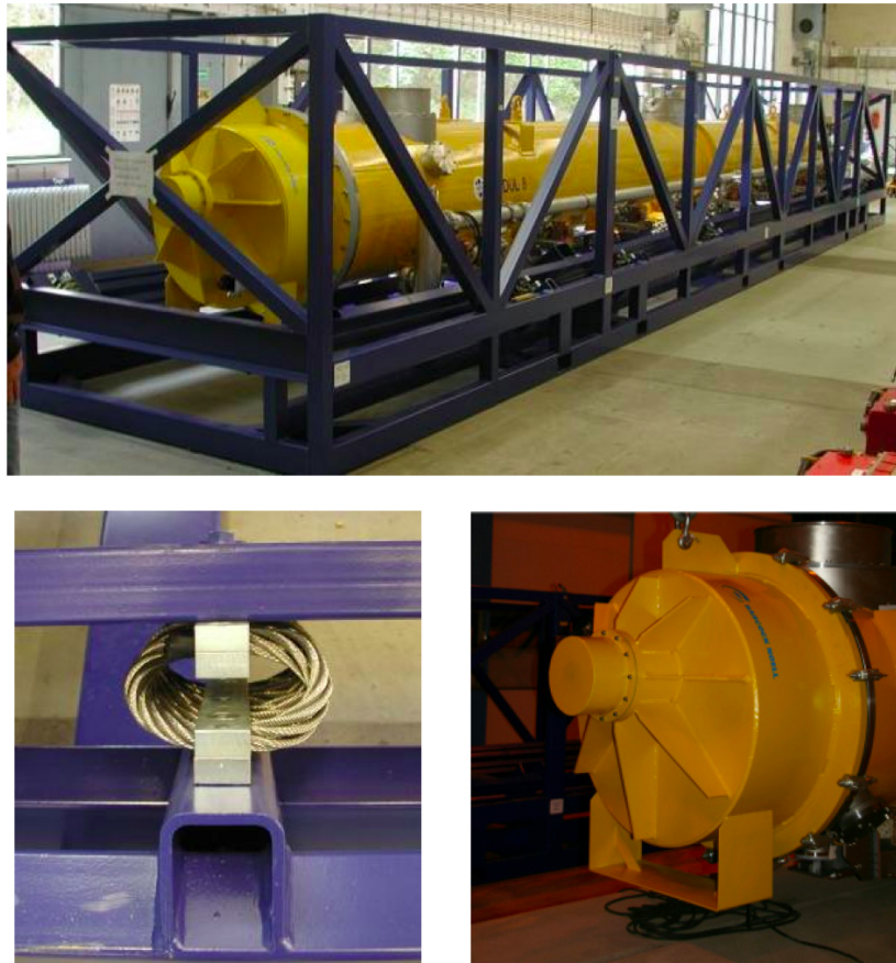
Figure 3.23. An European XFEL prototype cryomodule in its transport frame. The module is supported on vibration dampers [43]
