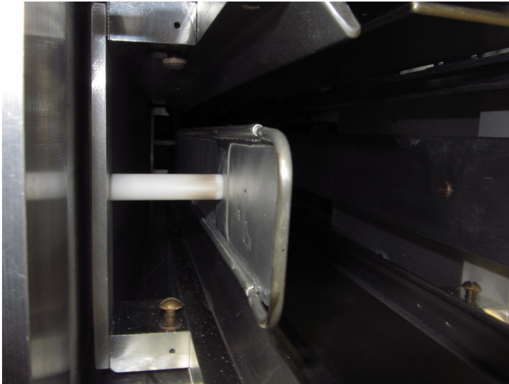
Figure 13.14: The side support insulators are varnished due to trapped electron obstruction during negative muon operations at BNL (darkened appearance close to the plate).
