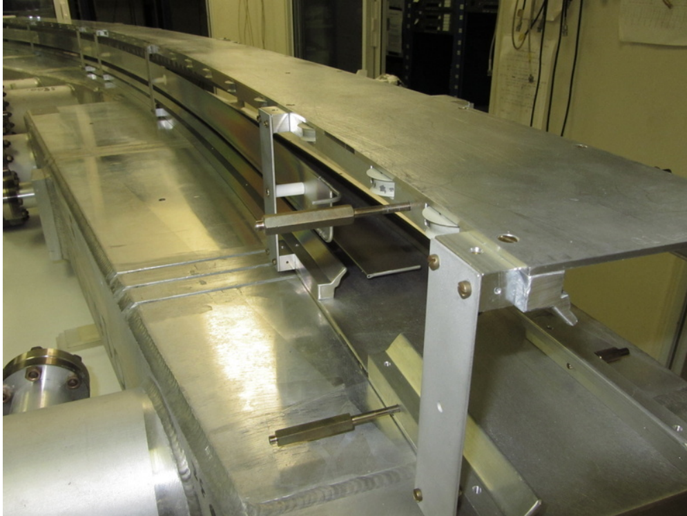
Figure 13.5: One cage (placed here up-side-down) that holds the plates of the electrostatic quadrupoles of the muon ( g - 2 ) experiment.
