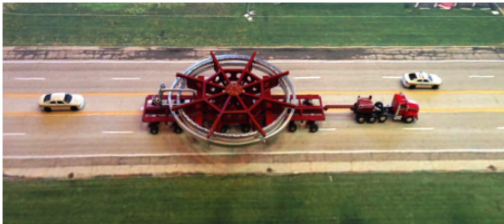
Figure A.4: Scaled model showing the specialized truck and trailer holding the coils.
