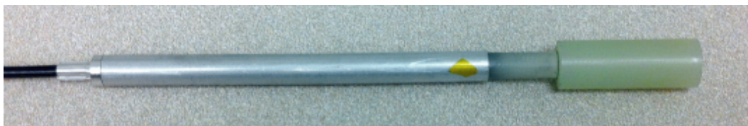
(b) pNMR probe with crimp connection
