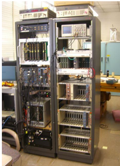
Figure 21.4: Photograph of the DAQ test stand including \mu TCA-based electronics and VME-based electronics at the University of Kentucky.
