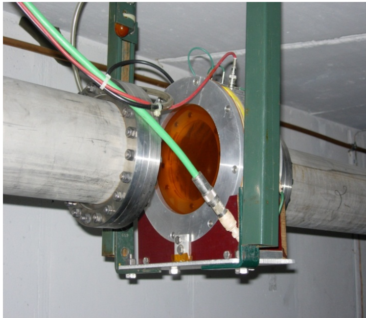
Figure 4.40: Fixed-position ion chamber in the AP2 line. The ion chamber is separated from the beam pipe by a vacuum window on each side. Fixed-position ion chambers will only be used in the M2 line. In locations like the M3 line and Delivery Ring that will also see Mu2e beam, the ion chambers will be put inside of vacuum cans and made retractable.
