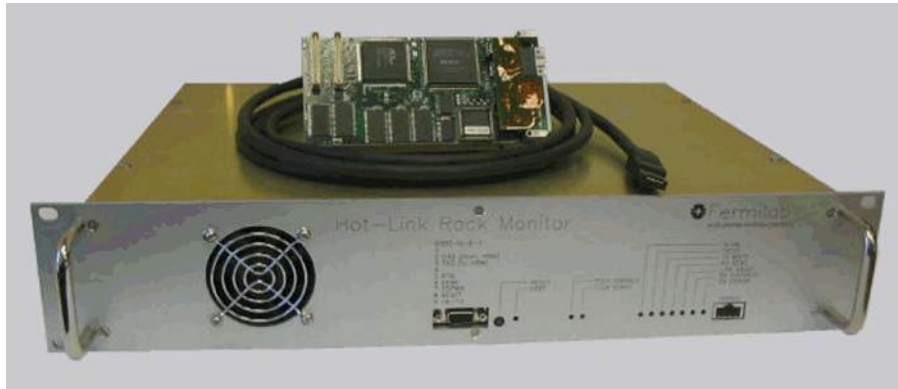
Figure 4.34: A Hot-Link Rack Monitor is a flexible data acquisition system composed of a remote unit and a PCI Mezzanine card that resides in a VME crate. Each HRM provides sixty four 16 bit analog input channels, 8 analog output channels, 8 TCLK timer channels and 8 bytes of digital I/O. HRM.s will eventually replace all of the functionality of CAMAC [20].
