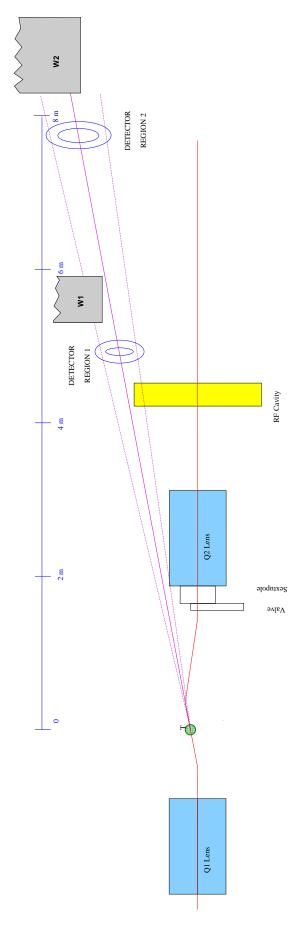
The RF cavity will be removed; it is not needed for VEPP-3 when the injection complex is operating. W1 (concrete wall) and Q2 (quadrupole FIG. 6. Top view at the VEPP-3 area close to the internal target equipment. Two possible locations of the photon detector are indicated. lens) will be machined around the VEPP-3 median plane to provide a free path for photons to the detector.
