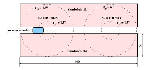
FIG. 8. The layout of the sandwich detectors
