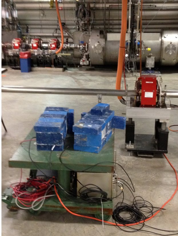
FIG. 19: Pb enclosures (blue) housing the two NaI/PMT detectors near the IR line. Cryo module FL02 is in the background.
