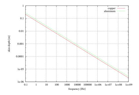
FIGURE 1. Skin depth versus frequency for copper and aluminum
