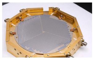
Figure 1: microwave kinetic inductance detectors array
