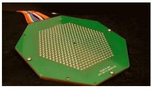
Figure 2: Hexagonal cryogenic wafer mapper based on light emitting diodes (LED).
