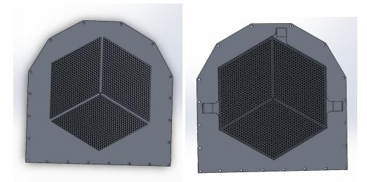
Figure 5 : Feedhorn Block, Designed by using Solidworks
