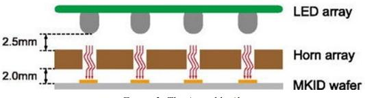
Figure 3: The Assembly Alignment
