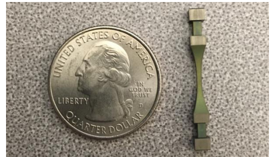
Titanium sample used for testing The dimensions of sample cross section: 1 mm x 1 mm.
