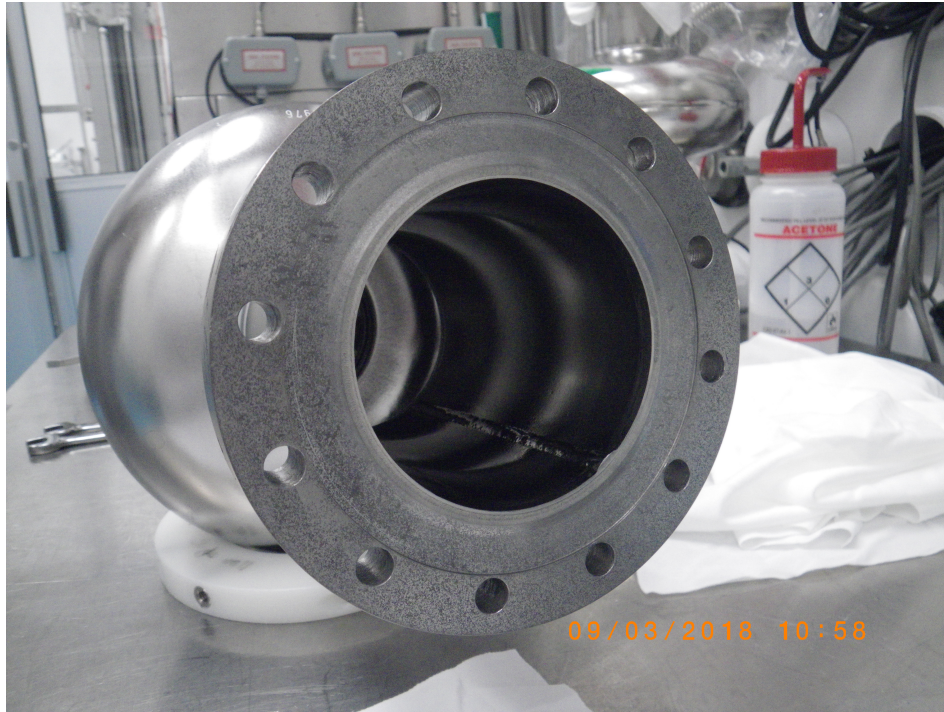
Figure 6.8: Black speckling was observed on the NbTi flanges of C7(N1) as well as C8(N1), pictured here.
