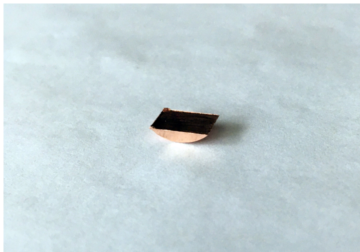
Figure 9.13: One of the copper shims used for mounting the instrumentation in the thermal finger assembly.
