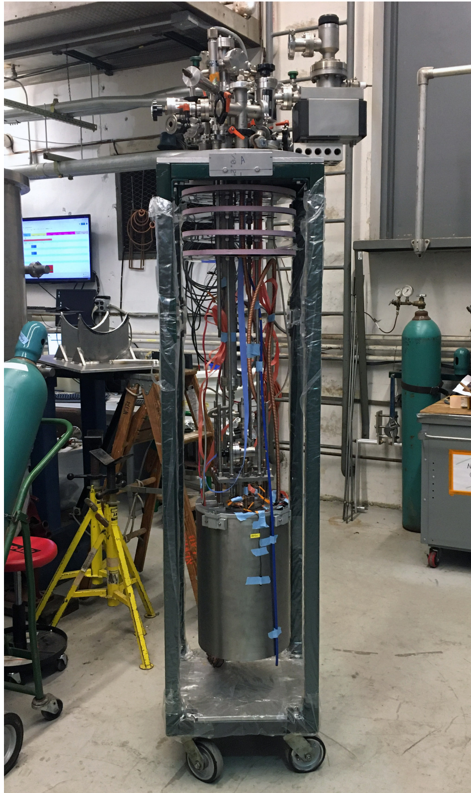
Figure 9.30: The DC Field Dependence Cavity installed on the vertical test insert with superconducting magnetic shielding can and external instrumentation.
