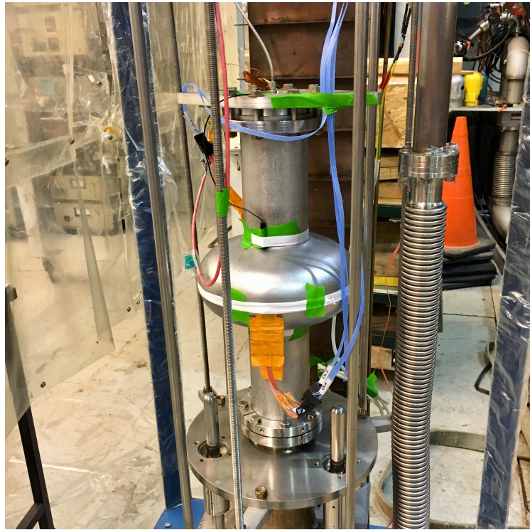
(b) Closeup of dressed cavity on insert
