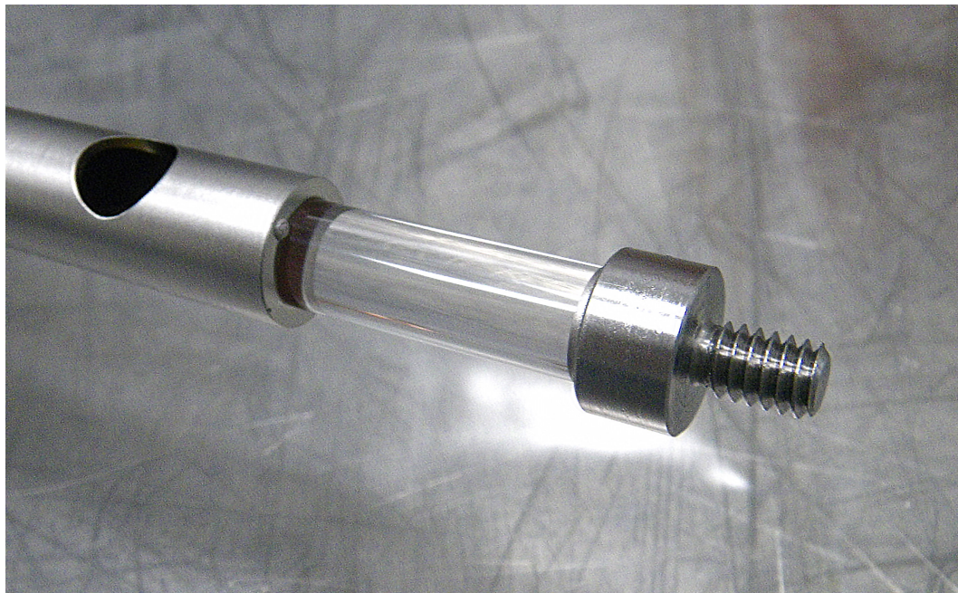
Figure 9.18: Close-up image of the sapphire rod installed in the thermal finger assembly.
