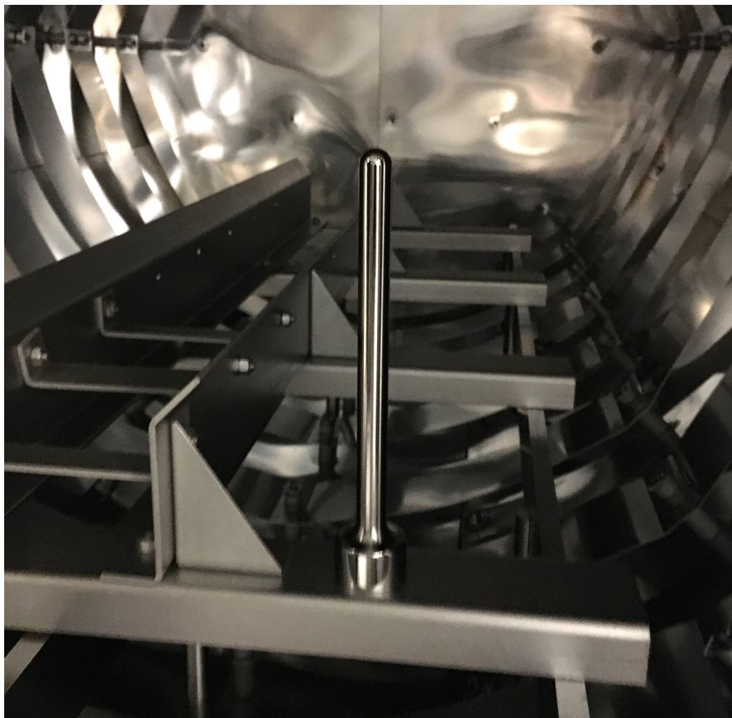
Figure 9.20: A niobium inner conductor sample for the DC Field Dependence Cavity installed in the vacuum furnace before an 800 °C degas bake.
