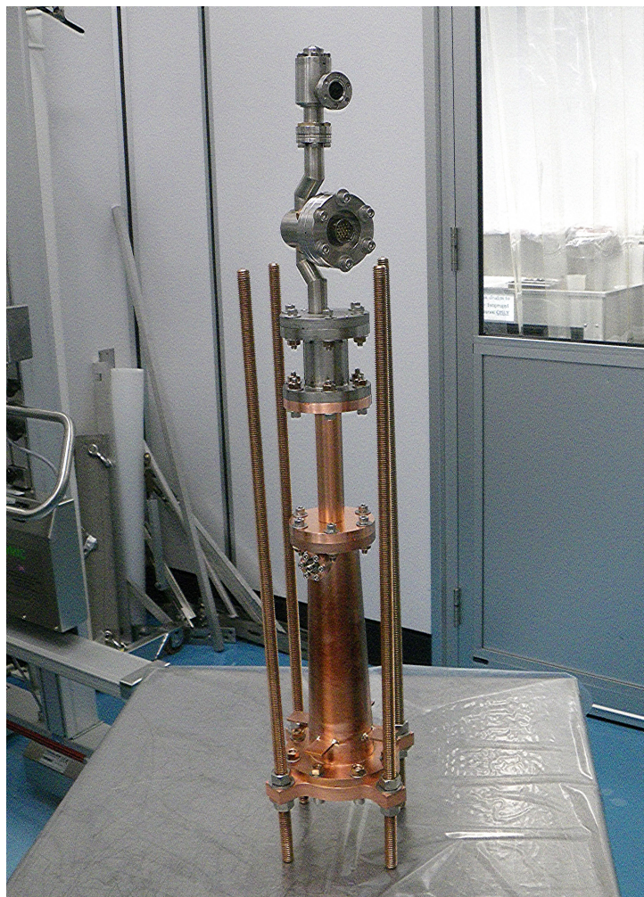
Figure 9.28: The fully assembled vacuum components of the DC Field Dependence Cavity apparatus with silicon-bronze support rods.
