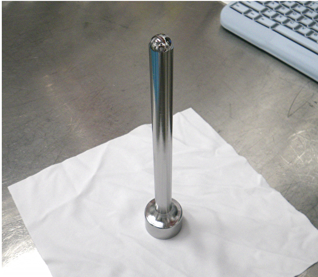
Figure 9.21: A niobium inner conductor sample for the DC Field Dependence Cavity after chemical processing and vacuum degas bake, just before assembly into the cavity.
