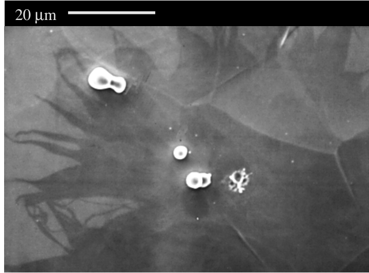
Figure 5.34: A field emitter found in a 5.8 GHz mushroom cavity. The previously molten iron particulate to the top left is too large to have been ejected by the craters, and it is likely that it was melted by the same plasma that produced the starburst.
