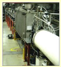
Energy upgrade cryomodule in the ATLAS tunnel.
