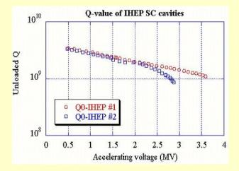
Vertical test results at KEK for two BEPC cavities.
