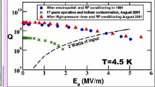
Argonne Split Ring Resonator, Frequency = 97 MHz,  $E_{\rho k}$  = 4.8 Eacc ,  $H_{p k}$  = 183 Oe/MV/m. Performance improved substantially after high pressure rinsing.
