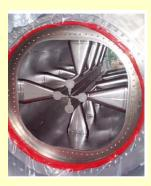
160 MHz medium beta PIAVE injector cryostat with Nb-Cu sputtered resonators. PIAVE extends the mass range of beams up to Uranium reaching 6 MeV/u of energy. In the very low  $\beta$  range from 0.01 to 0.05, the superconducting RFQ offers low power consumption for cw operation. Two structures delivered 4.7 MV in 2.13 m in PIAVE.
