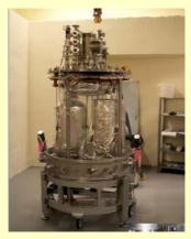
High beta cryomodule by Orsay.
