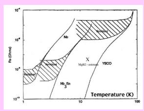
A comparison of superconductors Nb, Nb<sub>3</sub>Sn YBCO and  $MgB_2$  at 1 GHz.
