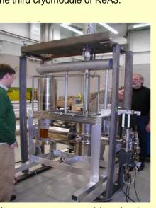
A prototype cryomodule housing a quarter-wave and a half-wave structure along with focusing magnets.
