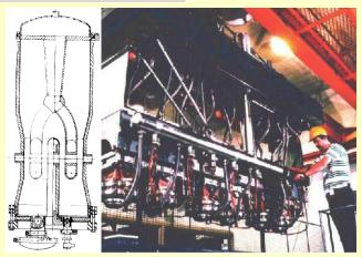
ATLAS Injector Cryomodule with inter-digital structures for particle velocities from 0.01c to 0.05 c (shown on left).
