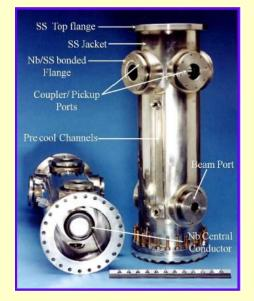
Completed resonator made from solid Nb and electron beam welding.
