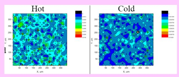
The hot samples show a high density of dislocations compared to the cold sample.
