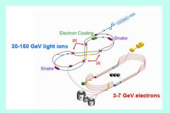
The Electron-Light-Ion Collider (eLIC) concept developed by Jlab.
