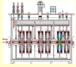
SARAF prototype module (PSM) with six HWR with  $\beta = 0.09$  for Phase I.
