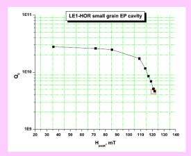
Electropolished single cell 1.3 GHz cavity with high field Q-drop.
