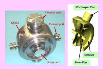
LANL,  $\beta$  = 0.175, 175 MHz, single spoke, 2-gap cavity.
