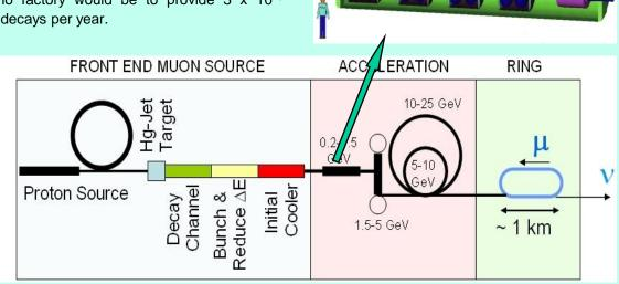
A generic neutrino factory from proton source to muon production, followed by cooling and acceleration. The demands on muon cooling are much reduced over that for a collider. In the final storage ring, muons decay to produce the desired intense neutrino beam.
