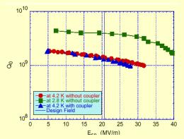
Performance of 500 MHz crab cavity The design kick is 1.44 MV, corresponding to peak surface fields of 21 MV/m and 60 mT.
