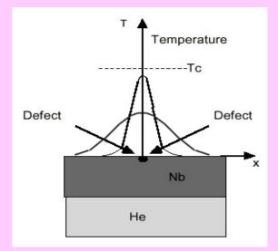
As the thermal conductivity improves, the defect and the niobium around it stay below the transition temperature. It becomes possible to raise the field further.
