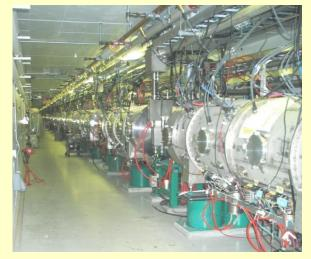
23 Cryomodules installed and operating at SNS.
