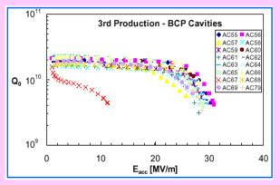
Performance of 9-cell cavities at DESY prepared by chemical etching, limited by high-field Q-drop.
