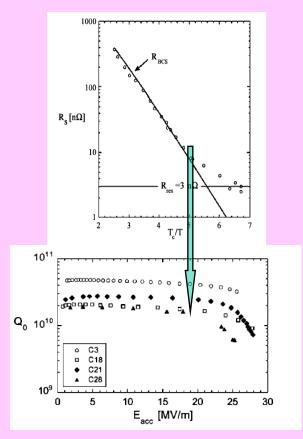
At 2 K, the BCS component of the surface resistance dominates the Q of  $2x10^{10}$  so that lowering the temperature to 1.8 K improves Q to  $5x10^{10}$ .
