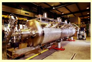
Superconducting cavities and cryomodules installed in the LHC, operating at an initial 7 TeV CM energy. At 400 MHz, 16 Nb-Cu cavities in 4 cryomodules provide 16 MV per beam and can deliver about 180 kW of beam power when needed. SRF cavities will help resolve the issue of transient beam loading by virtue of their low impedance and high cell voltage.
