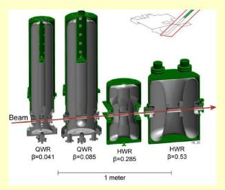
Resonator geometries for FRIB. There will be 335 of these resonators in two linacs.
