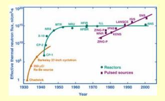
The highest intensity accelerator-based neutron sources in operation today are LANSCE at Los Alamos and ISIS at Rutherford Lab. The SNS at Oak Ridge National Lab is the first advanced pulsed spallation source with 1.4 MW of beam power at the target, upgradable to 5 MW. 6 Partner Labs: ANL, BNL, JLAB, LANL, LBNL, ORNL built SNS at ORNL in Oak Ridge Tennessee.
