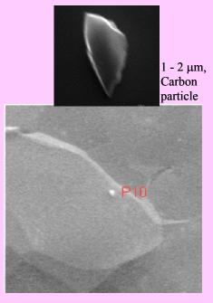
Typical field emitter, carbon micro-particle.
