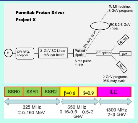
Schematic layout for the Fermilab Project X (formerly Proton Driver) SSR is single spoke resonator. ILC section has nearly ILC compatible cavities.
