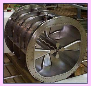
Superconducting RFQ for Injector PIAVE at INFN.
