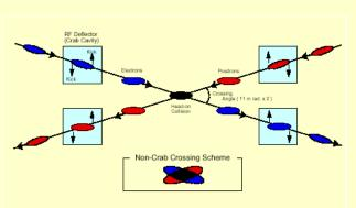
The crab crossing scheme allows a large crossing angle collision without introducing any synchrotron-betatron coupling resonances
