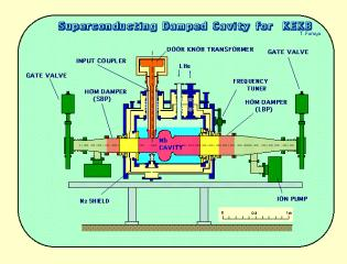
KEK-B cavity and cryomodule.
