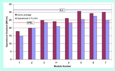
Steady advance in cryomodule gradients at DESY.
