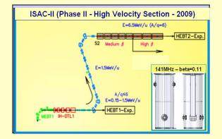
In the second stage (installation in 2010) another twenty cavities at  $\beta = 0.11$  (141MHz) will raise the final energy to 6.5 MeV/u, doubling the voltage gain of ISAC-II. The cavities will be housed in three cryomodules with six cavities in each of the first two modules and eight cavities in the third. Each cryomodule has one superconducting symmetrically solenoid placed in the cryomodule. Production of the cavities is with a Canadian company, PAVAC Industries of Richmond, B.C.
