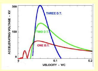
Non-relativistic ion beams require a broad velocity acceptance. The more drift tubes (D.T.) in a structure the more the total voltage gain, but at the cost of a smaller velocity range.
