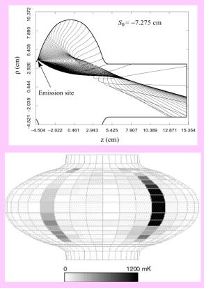
Temperature map showing a longitudinal heating profiles due to field emission.
