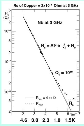
Surface resistance (Rs) vs. Temperature of niobium at 3 GHz, showing the exponential drop due to the energy gap.
