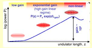
Micro bunches develop emitting photons coherently. The gain in power is exponential with undulator length until it reaches saturation at full bunching.
