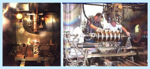
Electron beam welding at Cornell and JLAB.
