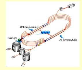
CEBAF is the largest SRF accelerator in operation in 2010. It has two 0.6 GeV linacs in the North and South tunnels, with 20 cryomodules each, and another 2<sup>1</sup>/<sub>4</sub> cryomodules in the injector making a total of 42<sup>1</sup>/<sub>4</sub> cryomodules. Each cryomodule has eight 5-cell cavities, making a total of 338 cavities. Having operated for more than 15 years it has accumulated more than 6 cryomodule-centuries of operating experience.
