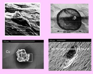
Typical examples of quench-producing defects located by temperature mapping and imaged by SEM are: chemical stains, foreign metal inclusions, pits with sharp edges, metal burrs from scratches, voids or delaminated regions of Nb, weld beads and other types of welding mistakes. 0.1 to 1 mm size defects cause thermal breakdown.
