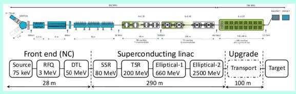
Schematic layout of ESS (European Spallation Source).
