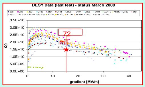
Distribution of 9-cell cavity performance from two vendors (measured at DESY).
