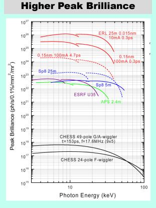
Cornell is proposing a synchrotron radiation light source as an extension to the CESR ring. The ERL will be driven by an energy recovering SRF linac operating at an energy of 5 GeV and an average current of 100 mA. While offering average photon flux comparable to storage rings, the proper parameters of an ERL can lead to higher peak brilliance, shorter pulses and a higher coherent fraction. The Cornell ERL will need 350 cavities and 60 cryomodules. KEK is proposing a similar 2.5 – 5 GeV ERL.
