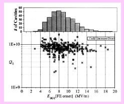
Distribution of gradients and  $Q_0$  at the onset of field emission for more than 300 CEBAF cavities tested in the early 1990's. The average gradient is 8.7 MV/m.
