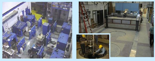
Vertical Cavity Testing at JLAB and Cornell.
