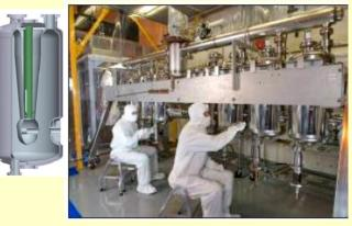
ATLAS energy upgrade cryomodule with seven  $\beta = 0.15$  structures (shown on left). The average accelerating gradient is 11.7 MV/m.
