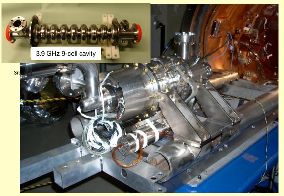
3.9 GHz cavity package showing 9-cell cavity in its helium-vessel, tuner, support and alignment, ready to be installed in a horizontal test cryostat at Fermilab.
