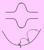
The spherical or elliptical shaped cavity eliminates multipacting.
