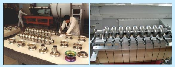
9-cell cavity fabrication and mechanical quality control at DESY.
