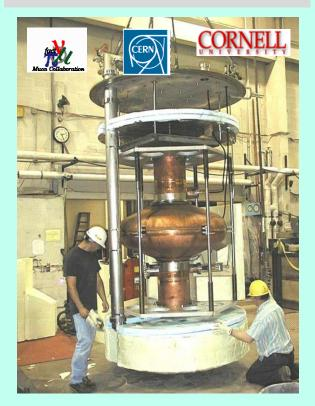
A CERN-Cornell collaboration designed, fabricated and tested a 200 MHz single cell Nb-Cu cavity. In the first such unit, an accelerating field of 10 MV/m was reached at a Q near 10<sup>9</sup>. The neutrino factory and the muon collder call for several hundred meters of 200 MHz cavities to provide gradients of 15 MV/m. Nb-Cu is the technology of choice driven by the cost concern. The success of 400 MHz LHC cavities in reaching comparable gradients is encouraging.
