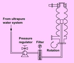
A jet of ultra pure water dislodges surface contaminants that normally resist removal with conventional rinsing procedures. The benefits of HPR in reducing field emission are well demonstrated in tests with multicell cavities that reach accelerating fields of 35 MV/m at DESY.
