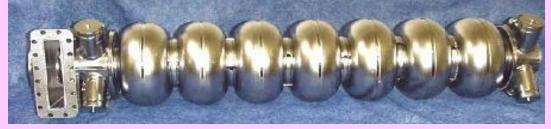
JLAB upgrade 7-cell Low-Loss cavity for lowering H<sub>pk</sub>.
