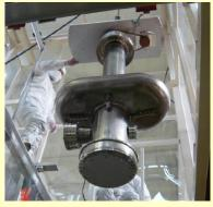
The crab cavity is 1m by 0.5m in cross -section.
