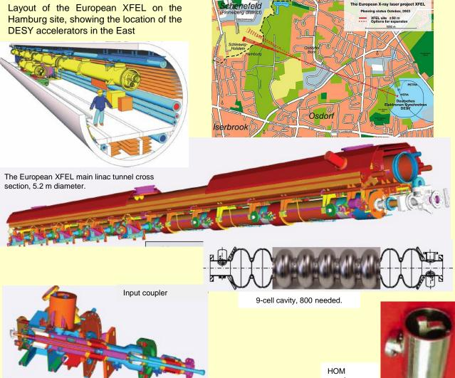
The main linac will have twelve meter long accelerator modules with 8 superconducting cavities each, grouped into about 20 rf stations. The linac will be housed in a tunnel 15 to 30 m underground. The required klystron power per station is about 5 MW,
