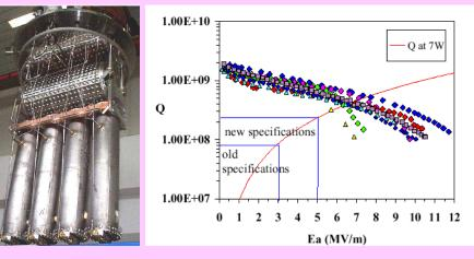
INFN Injector PIAVE 80 MHz Quarter-Wave Resonators beta = 0.05.
