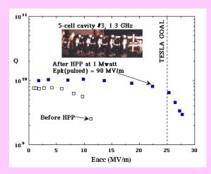
An example of ``before-and-after" HPP. Here a cavity contaminated down to 10 MV/m improves with HPP to 28 MV/m.
