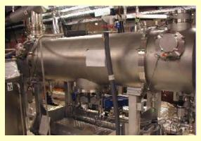
Rossendorf Cryostat, with two 9-cell cavities based on TELSA technology.
