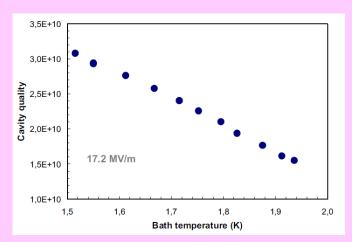
High Q values for a 9-cell cavity measured in the BESSY test cryomodule.
