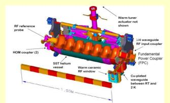
The CEBAF Upgrade cavity package, coaxial HOM couplers outside the He vessel, waveguide fundamental power coupler, and scissors type tuner.
