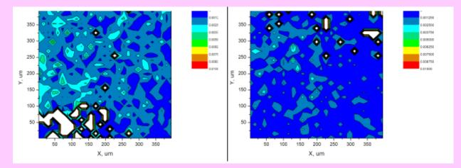
Baking at 120 C for 48 hours significantly reduces the dislocation density of both the hot and cold samples.
