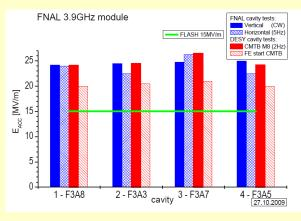
Performance results comparison for vertical test, horizontal test at FNAL, and cryomodule test at DESY.
