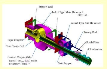
3D layout of the crab cavity in its helium vessel .
