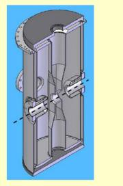
(Left) 3D schematic of a Half-Wave resonator (HWR). (Right) 176 MHz,  $\beta = 0.09$  HWR built for SARAF by ACCEL. The resonator height is 85 cm.
