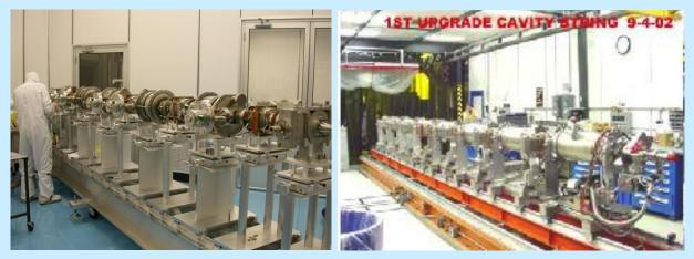
ERL-injector cavity string assembly at Cornell.
