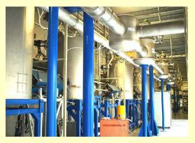
Inside ALPI at INFN Legnaro. ALPI has been in operation since 1994. In all, 64 QWR at 160 MHz are in the main beam line delivering a total of 49 MV. 44 cavities are medium  $\beta$  (0.11) and 8 are high  $\beta$  (0.13). 12 low  $\beta$  (0.055) resonators at 80 MHz are made from solid Nb. Both Nb and Nb-Cu resonators reached 6 to 8 MV/m at 7 watts in vertical tests.
