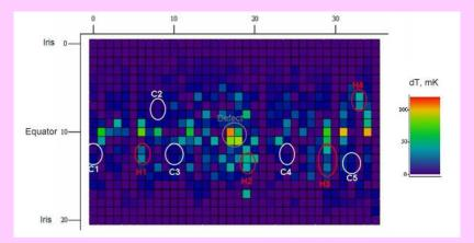
Temperature map of a single cell cavity with high field Q-drop shows regions of strong heating (hot spots) and regions of weak heating (cold spots) in the high magnetic field.
