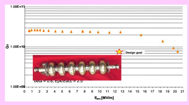
$\beta = 0.8$ , 805 MHz, Epk/Eacc = 2.5, tested at JLAB.
