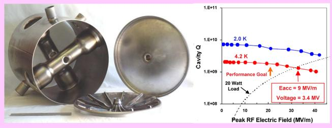
Argonne, 345 MHz ,  $\beta$  = 0.4, double Spoke Resonator.
