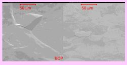
Comparison of a niobium surface prepared by (left) standard chemical polishing and (right) electropolishing.
