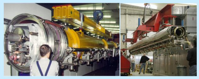
Cryomodule assembly at DESY.
