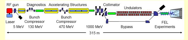
FLASH: One GeV linac for SASE FEL to 6.6 nm.
