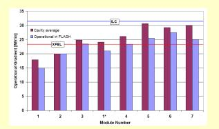
Evolution of cryomodule gradients over installation history. The bar chart compares linac and cavity acceptance test results. The average degradation is a few MV/m. Module 6 has only cavities prepared by the latest techniques of electropolishing and baking.
