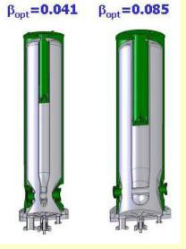
Quarter wave resonator designs for ReAccelerator3.
