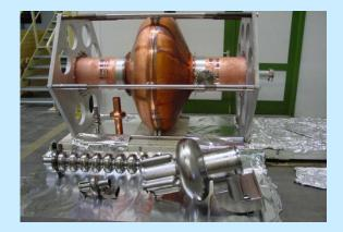
A variety of superconducting cavities for accelerating velocity-of-light particles. In the foreground (left) is the 9-cell cavity and (right) a CESR 500 MHz cavity together with a 1/3-scale version of the latter. In the background the large 200 MHz Nb-Cu cavity dominates. With a few micron layer of niobium sputtered on the inside, the cavity was developed by a Cornell/CERN collaboration for future muon accelerators and the neutrino factory.
