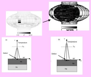
(Above) Temperature maps of a single cell cavity show spot heating as a precursor to large region of the cavity becoming normal conducting when the quench develops.
