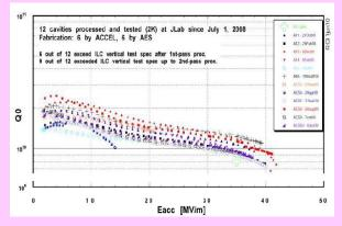
Performance of twenty-four 9-cell electropolished and baked (120C) cavities at DESY and JLAB reach 40 MV/m with no Q-drop.
