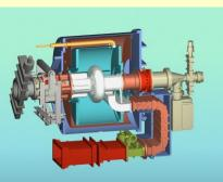
CESR cavity and cryomodule.
