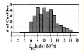
Usable gradients for CEBAF cavities at first installation. Most of the 42 cryomodules have been kept permanently cold since 1995. From October 2000 through June of 2001, CEBAF delivered more than 4500 beam hours for physics. SRF cavity related faults accounted for less than 0.5% down time. Cavity gradients are being steadily upgraded by re-processing from 7 to 15 MV/m.
