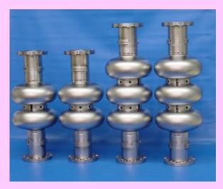
Two and three cell cavities hydroformed at DESY.
