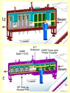
Cryomodule layouts for the QWR and HWR resonators. There will be 45 cryomodules in all.
