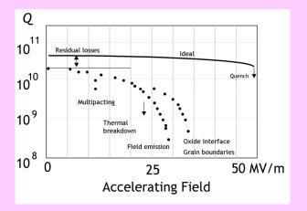
Ideally we would expect the cavity *Q* to remain constant (at the BCS predicted value) as the field increases, until the quench field. However, as surface electric and magnetic fields rise, several effects set in to drop the *Q*. These are multipacting, thermal breakdown, medium field slope, field emission, and high field *Q*-drop. Most of these effects are now understood and solutions invented.
