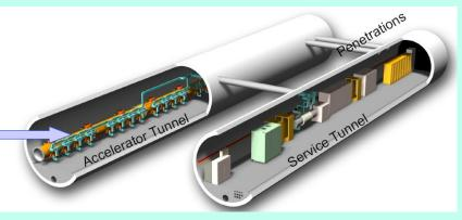
Two tunnel layout for the ILC, one for the accelerator and second for the RF sources and other services.
