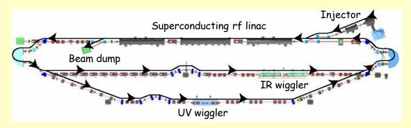
Layout of the Jlab IR FEL with UV upgrade. The FEL runs in the energy recovery mode. It comprises a 10 MeV injector, a linac consisting of three Jefferson Lab cryomodules generating a total of 80 to 160 MeV of energy gain, and a recirculator.
