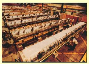
350 MHz Nb-Cu 4-cell cavities and cryomodules. More than 270 cavities were installed. Nb-Cu cavities will play an important role for low frequency cavities (100 – 350 MHz), such as those needed for a future neutrino factory, or muon collider
