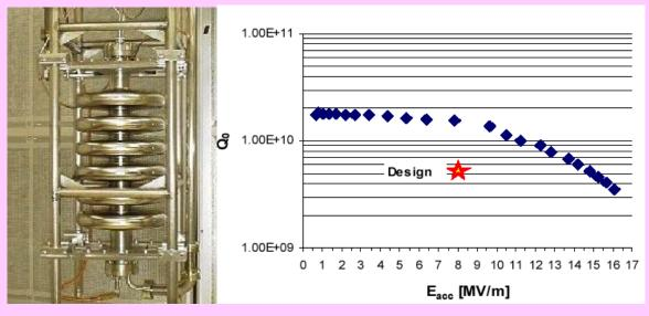
MSU,  $\beta$  = 0.49, 805 MHz, e-beam welded and tested at JLAB.
