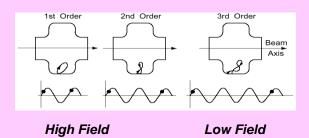
In the early stages of SRF development, prior to 1980, a major performance limitation was ``multipacting." 1.3 GHz structures were limited to about 3 - 4 MV/m.
