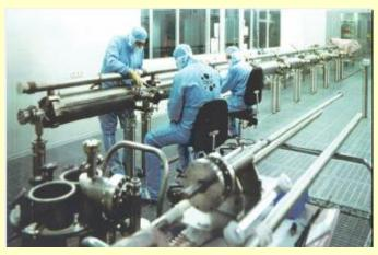
Cavity string assembly in clean room at DESY.
