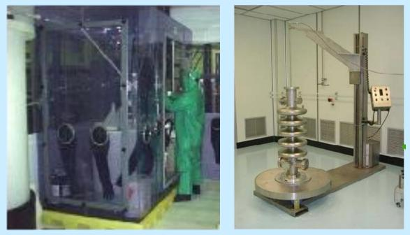
Chemical Treatment at MSU and high pressure rinsing at Los Alamos.
