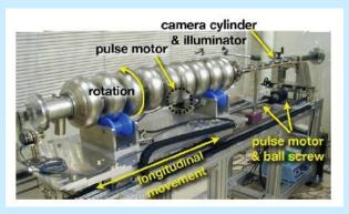
Internal cavity inspection system at KEK with CCD camera.
