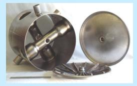
345 MHz,  $\beta$  = 0.4, double-spoke resonator (ANL) The presence of a spoke through a TM cavity makes the structure both compact and rigid, allowing low frequencies.
