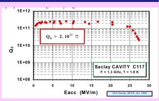
The world-record Q value is  $2x10^{11}$  for a single cell 1.3 GHz cavity at 1.6 K and an ambient magnetic field less than 5 mGuass.
