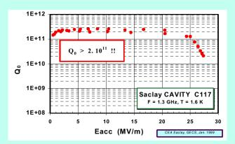
In some of the best performing cavities, Q values of 10<sup>11</sup> have been reached in 1.3 GHz single cell test cavities at 1.6 K and accelerating fields of 25 MV/m. The corresponding energy decay time is of the order of 10 seconds!
