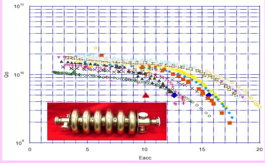
$\beta$  = 0.61, 805 MHz, Epk/Eacc = 3.5, tested at JLAB.
