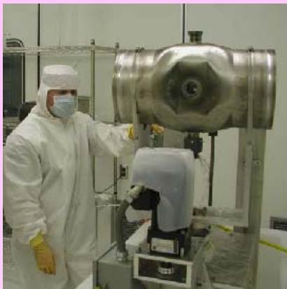
MSU, half-wave resonator, beta = 0.285, 322 MHz
