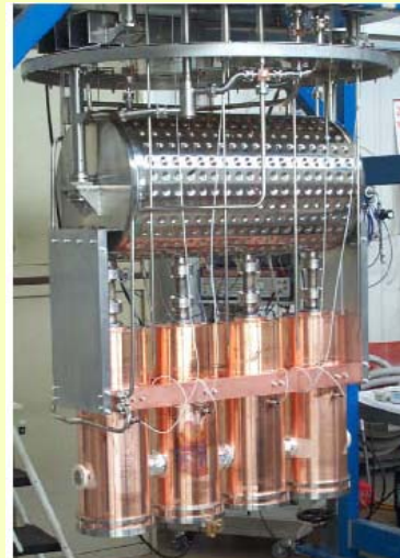
160 MHz medium beta PIAVE injector cryostat with Nb-Cu sputtered resonators. PIAVE extends the mass range of beams up to Uranium reaching 6 MeV/u of energy.
