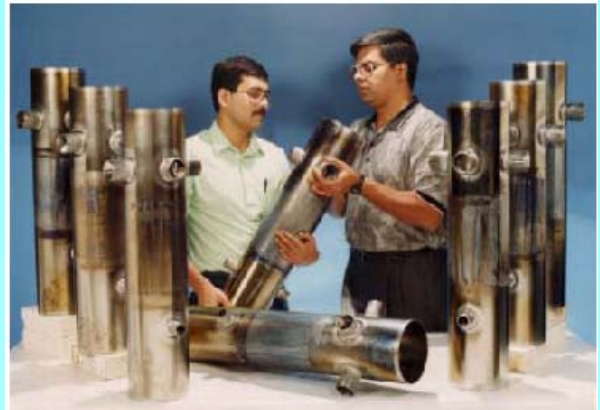
Resonator Fabrication at ANL
