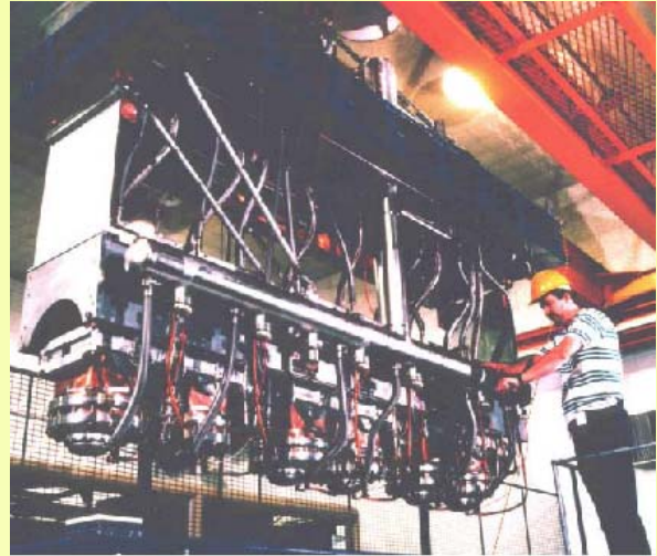
ATLAS Injector Cryomodule
