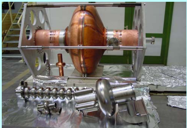
Prototype 1500 MHz, 7-cell cavity for CEBAF upgrade
