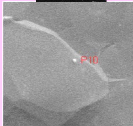
Typical field emitter, carbon micro-particle
