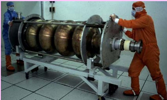
CERN Nb-Cu Cavity at 350 MHz
