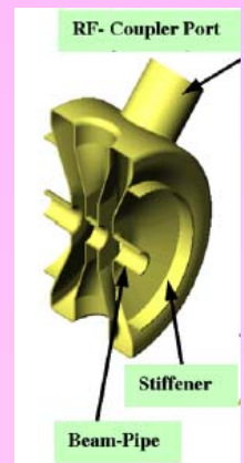
LANL, \beta = 0.175 , 175 MHz, single spoke, 2-gap cavity
