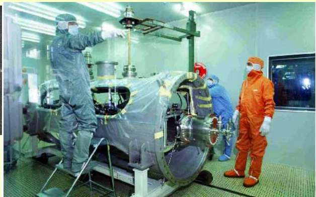
Nb/Cu single-cell HOM damped 352 MHz cavities, designed and built by a Saclay/CERN, collaboration were high power tested at ESRF to Eacc of 7 MV/m and transferred 360 kW to 170 mA beam.
