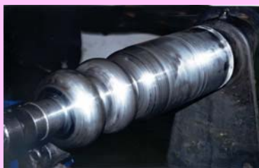
Spinning from a disk at INFN
