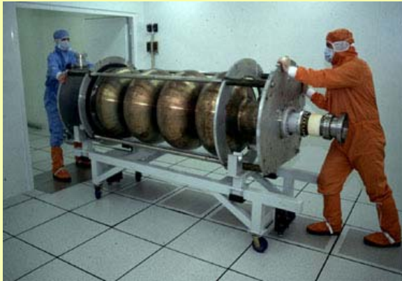
LEP-II 350 MHz Nb-Cu cavities and cryomodules
