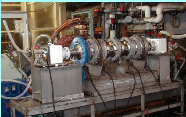
Electropolishing at KEK and DESY
