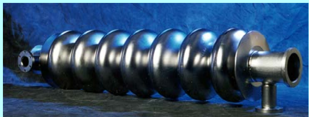
Prototype 1500 MHz, 7-cell cavity for CEBAF upgrade
