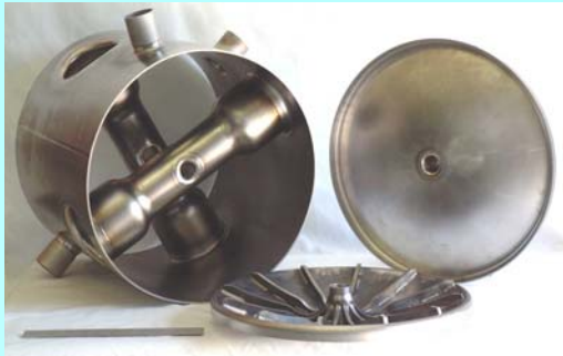
\beta = 0.47 , 800 MHz, 6-cell elliptical-cell (JLAB/MSU)
