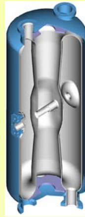
172.5 MHz, \beta = 0.14 Half Wave Resonator
