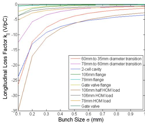
Figure 4: (color) Loss Factors for individual components as a function of bunch length as computed by NOVO.
