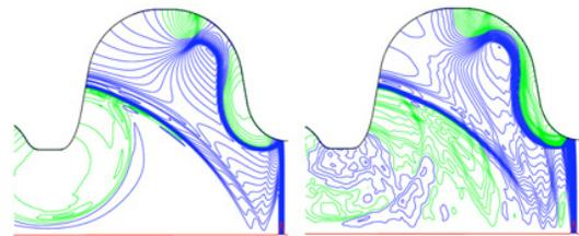
Figure 6: Comparison of electric force lines computed by NOVO for a bunch entering the two-cell cavity after also traveling through the beam entrance section of the cryomodule (left) and after just traveling through the 2-cell cavity in isolation (right).
