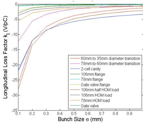
Figure 3: (color) Loss Factors for individual components as a function of bunch length as computed by ABCI.
