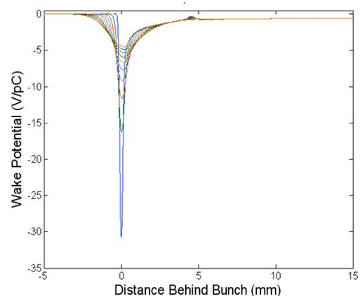
Figure 2: (color) Wake potential computed by ABCI for the 2-cell cavity at bunch lengths ranging from 0.1 mm to 1.0 mm. Shorter bunches result in a deeper potential well.
