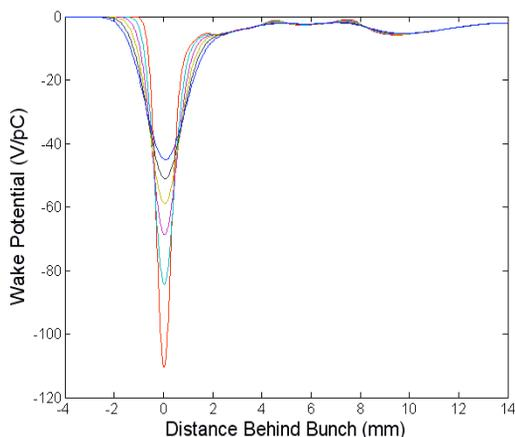
Figure 7: (color) Total wake potential the entire beam line of the injector cryomodule, as computed by adding individual wake potentials for each component, as computed by ABCI, for bunch sizes ranging from 0.1mm to 0.8mm.
