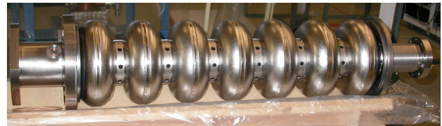
Figure 1: 7-cell cavity after final electron-beam welding.
