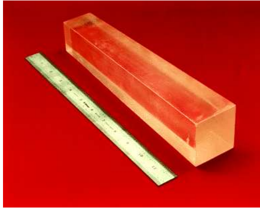
Figure 4.16: Photo of a single CsI crystal, 7800 of which are used in the crystal calorimeter.
