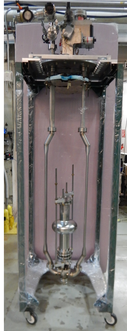
(b) Picture of the test stand after cavity assembly.
