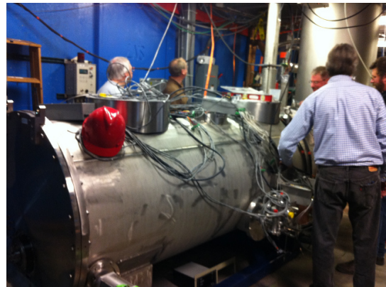
(f) The HTC being connected to the HEX can in the testing area.
