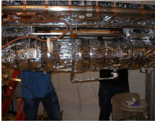
Figure 8.25: Picture of the solenoid around the cavity in HTC9-2.
