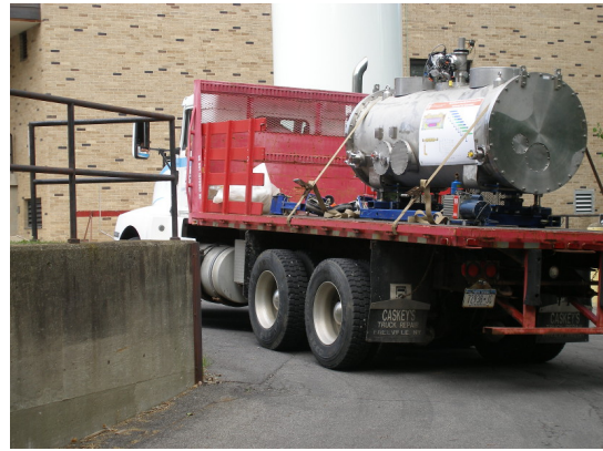
(d) The completed HTC on a truck for transport to the testing area.
