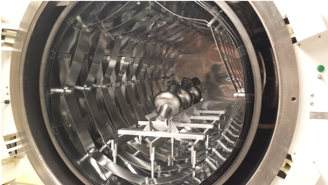
Figure 4.7: The Cornell UHV furnace with three single-cell ILC shaped cavities after a nitrogen-doping.
