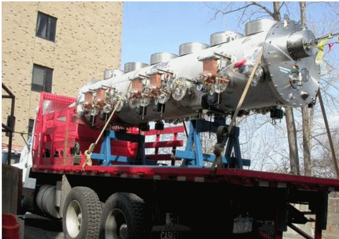
Figure 2.3.39: Transport of the completed ERL injector prototype cryomodule from the Cornell Newman Lab assembly area to the Wilson Lab test area.
