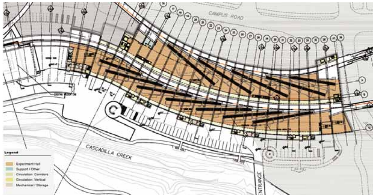
Figure 4.3.3: East building addition at 827' elevation, showing twin Linacs and 12 x-ray beam-line capability.
