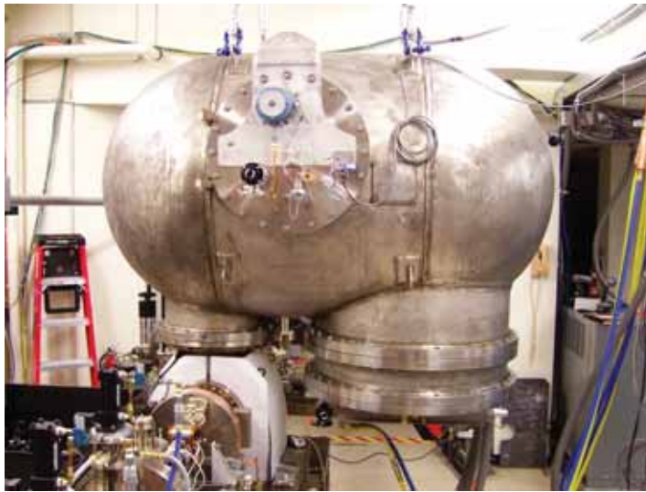
Figure 2.3.5: The Cornell gun with its SF 6 pressure vessel mounted. The HV power supply is mounted in the port to the right of the gun.
