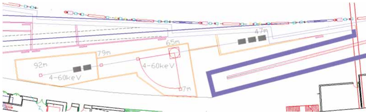
Figure 3.4.7: Floor plan for coherent diffraction beamline including an optics enclosure and two experimental hutches, both designed to allow use of the undulator's fundamental and higher harmonics. The first experimental hutch includes a diffractometer with a 7 m long detector arm that can be positioned in the horizontal plane. The detector arm in the forward-scattering direction will be 15 m. Experiments can be prepared in the second hutch while the first hutch is in use.
