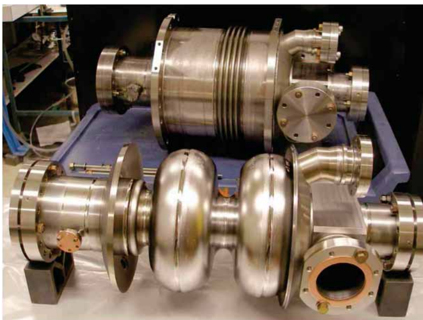
Figure 2.3.20: 2-cell cavity before and after welding the helium vessel
