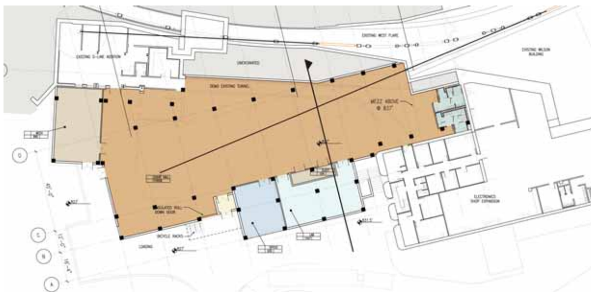
Figure 4.3.6: G-line Annex at level 827. The building contains a long undulator beamline from a 25 m long ID and a new mechanical room to serve the annex and existing G-line.
