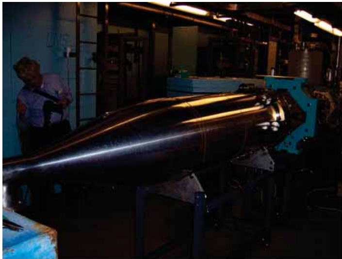
Figure 2.8.2: The completed Phase 1a beam stop before installation of its shielding.
