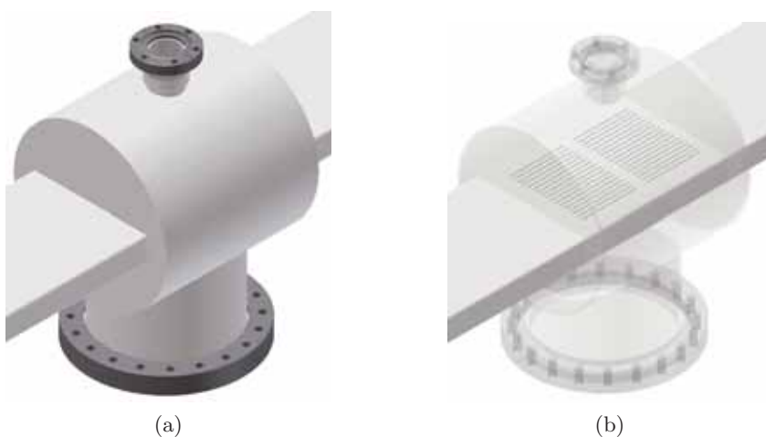
Figure 2.2.6: Lumped pumps are installed at pump ports comprising a shroud (Fig. 2.2.6a) welded around the extrusion with pumping slots and (Fig. 2.2.6b) cutting through both top and bottom.
