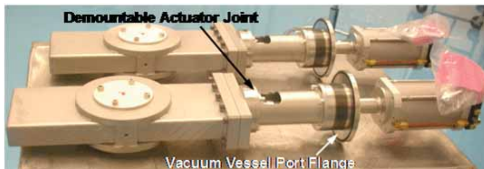
Figure 2.4.31: Cryogenic and RF rated pneumatic gate valves for the beamline.
