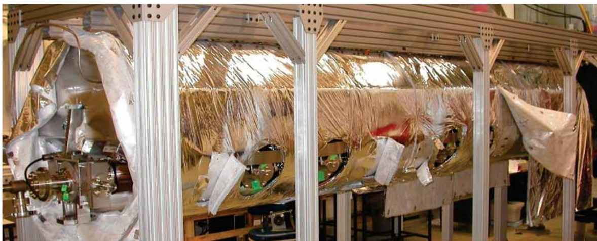
Figure 2.4.37: Photograph of the completed ERL Injector 100 K shield being wrapped with MLI.
