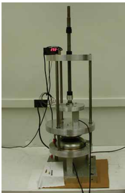
Figure 2.4.16: RF measurement set-up to determine the dumbbell trimming. This individual trimming process ensures a proper compensation of the small shape variations, leading to an almost perfect cavity after all fabrication steps
