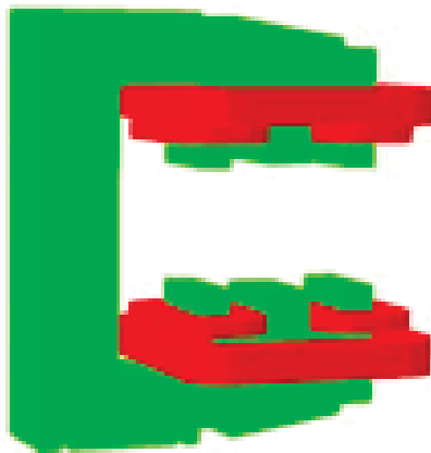
Figure 2.6.7: 3D depiction of the NSLS2 156 mm combined correction magnet that can be emulated in the ERL.
