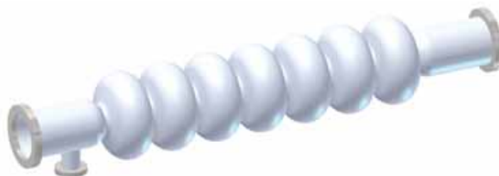
Figure 2.4.5: CAD model of the 7-cell ERL main Linac cavity.
