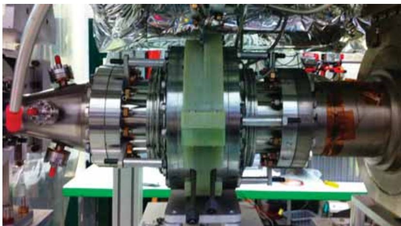
Figure 2.4.21: HOM absorber installed under the HGRP within the HTC cold mass
