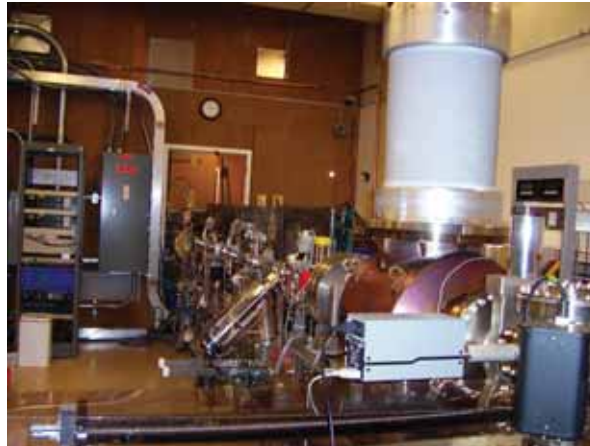
Figure 2.3.4: The developmental gun at Cornell, without its HV power supply and SF 6 tank, followed by the initial test beamline. The load-lock system is on the right rear of the gun.
