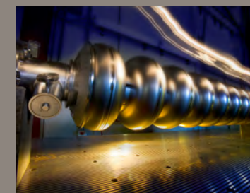
Building SRF Cavities
