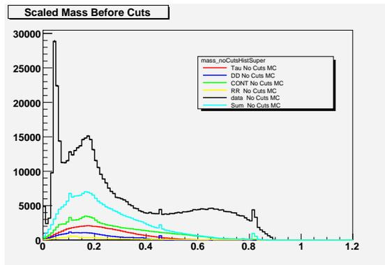
FIG. 1: Number of events vs. mass scaled to center of mass energy ( $E_{cm}$ ) BEFORE any cuts. Note  $D \rightarrow K\pi$  at 0.45 GeV and  $\gamma\psi' \rightarrow \psi$  at 0.8 GeV. Also shown is an unknown source of background for mass less than 0.1 GeV.
