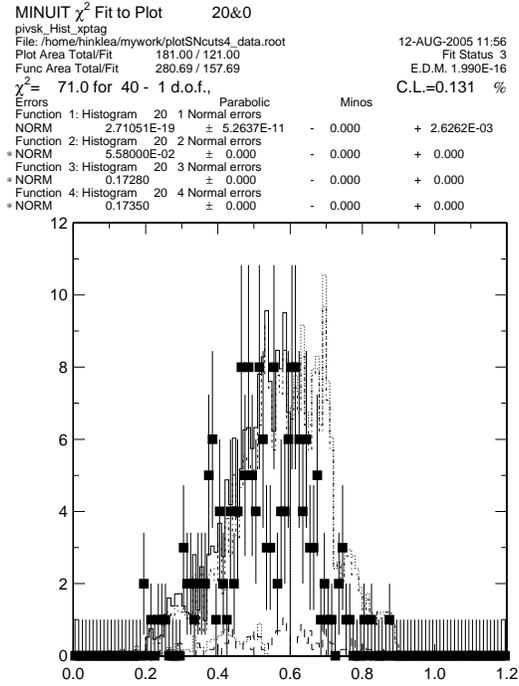
FIG. 25: Best fit of  $\pi^+vs.k^-$  with respect to tag momentum. This is a very poor fit. Very few tau events and a large number of background events are shown. This indicates that the tau rarely decays to kaons. This histogram was NOT included in the above eight when the cross-section was determined.
