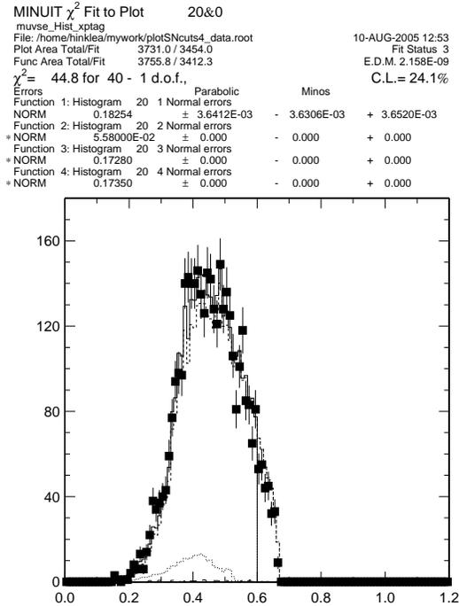
FIG. 20: Best fit of  $\mu^+vs.e^-$  with respect to tag momentum.
