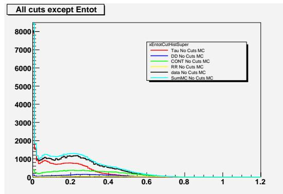
FIG. 5: Number of events vs. total neutral energy (GeV) with all cuts applied except the total neutral energy of the tracks
