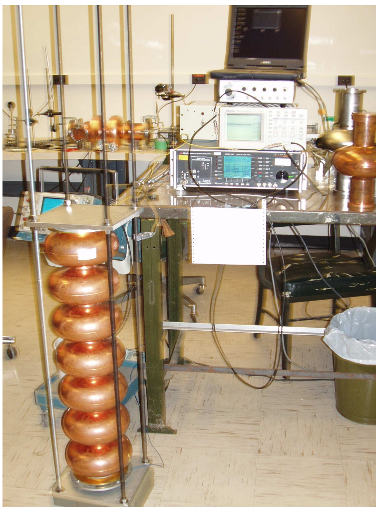
FIG. 7: Experimental Setup: scanning for resonances of a Cu 7-cell cavity. The cavity is shown lower left, with the data acquisition equipment on the table on the right.
