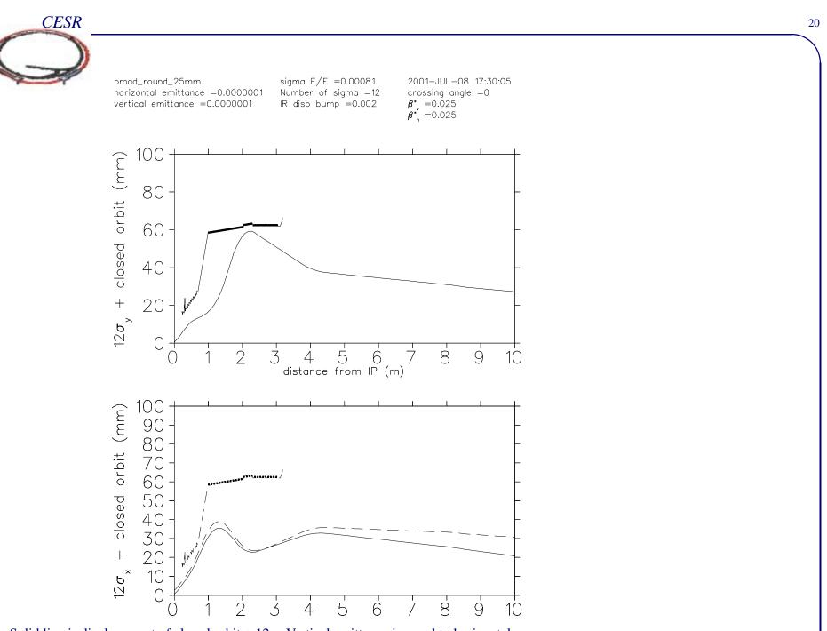
Solid line is displacement of closed orbit +  $12\sigma$ . Vertical emittance is equal to horizontal.
