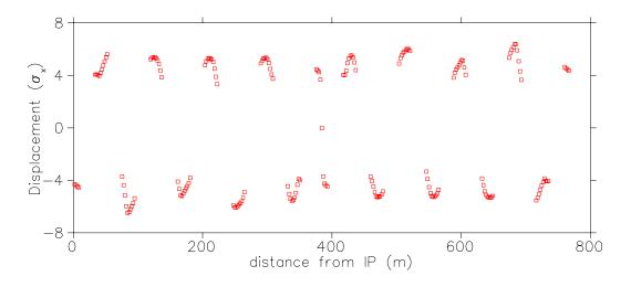
Separation at parasitic crossing points in units of horizontal rms beam size
