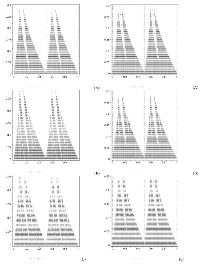
Figure 1: Stability diagrams for  $\lambda=0.00$ . Resonances up to second (A), fourth (B) and sixth order (C), respectively, have been included. The horizontal axis refers to  $\nu_0$  and the vertical axis refers to  $\xi$ .
