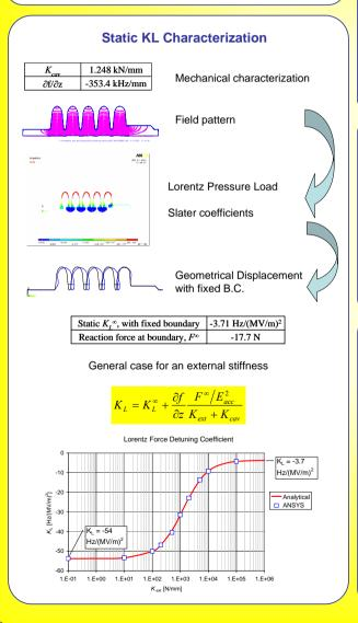
Parameter Value 704.4 MHz Design Frequency 0.47 Geometrical B ris radius 40 mm Cell to cell coupling 1.34 % 180 Ohm R/Q 160 Ohm 3.57 peak/Ea 5.88 mT/(MV/m) B<sub>peak</sub>/E<sub>acc</sub> 70 mm Stiffening ring radial position -3.7 Hz/(MV/m) Lorentz Force Coefficient (estimated)
