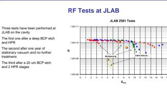
In Test #1 the cavity showed a easily conditioned multipacting level at low field and a barrier at 7-8 MV/m which needed long RF conditioning times.
