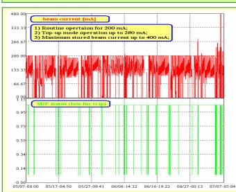
In May, there are totally two srf trips in user shifts due to LN2 flow rate too high and quench when beam loss suddenly. In June, there are totally two srf trips in user shifts due to false alarm of window arcing and poor contact of tuner force circuit socket. The other srf "trip" happened during machine maintenance (5% of machine operational time) and machine study shifts (19%) owing to access of srf radiation area, srf interlock check after system modifications, quench during beam loss, etc.
