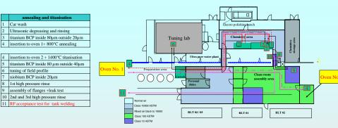
Workflow inside DESY cleanroom for cavity preparation => ANNEALING and TITANIUM POST PURIFICATION
