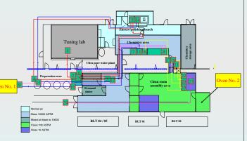
Workflow inside DESY cleanroom for cavity preparation => ELECTRO-POLISHING
