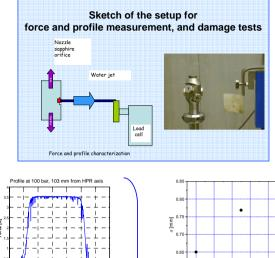
Assuming a gaussian profile for the water jet, we determine the force and the spot size interpolating the measured data with the following expression
