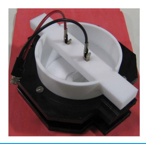
The EP setup for small samples is very simple and allows to have a good control on all fundamental parameters. Voltage drop, current, temperature of acid and temperature of water are monitored using in parallel: a strip chart analog recorder and a USB NI DAQ connected to a laptop. Data are acquired using a NI LabView custom application. The most complicated parameter to quantify is the acid agitation obtained with a magnetic stir bar . Current voltage characteristics as a function of temperature
