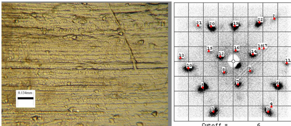
FIG. 6: sample 2 after plastic deformation and 900 C heat treatment for 1 hour and back reflection Laue method pattern
