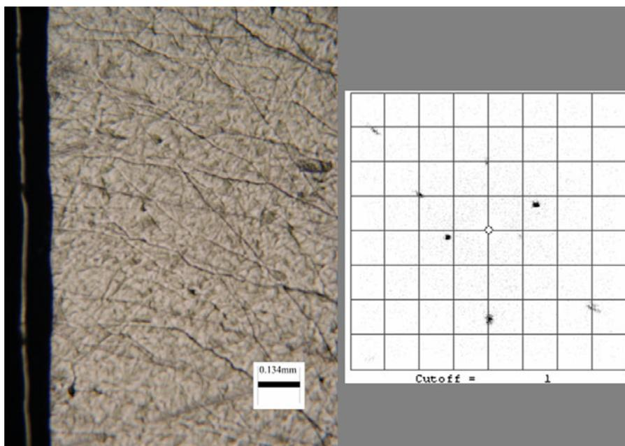
FIG. 10: heat affected zone with defects after EBW process and back reflection Laue pattern
