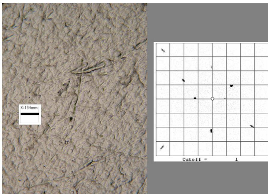
FIG. 9: non heat affected zone after the EBW process with back reflection Laue pattern
