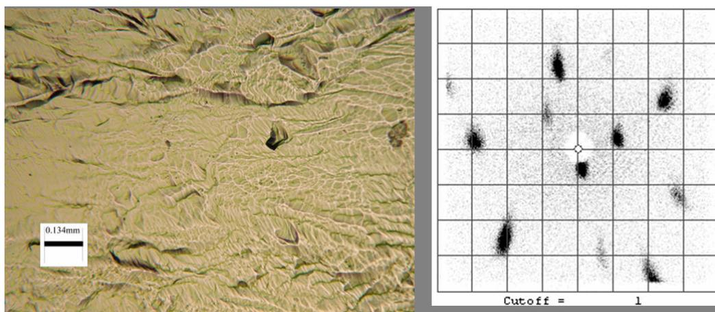
FIG. 4: sample 2 after plastic deformation and back reflection Laue method pattern
