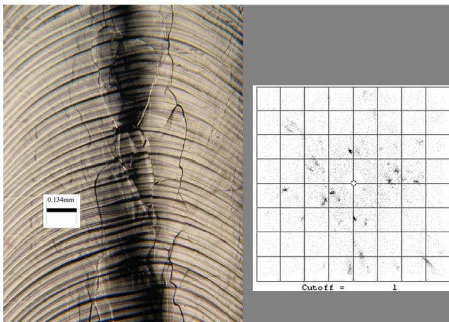
FIG. 11: welded region of two single crystals of niobium with re-crystallization into poly crystal and back reflection Laue pattern
