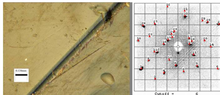
FIG. 1: sample 1 with known grain boundary, back reflection Laue method pattern taken from above grain boundary
