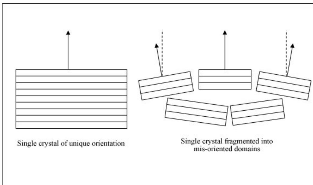
FIG. 5: visual representation of fragmented single crystal niobium
