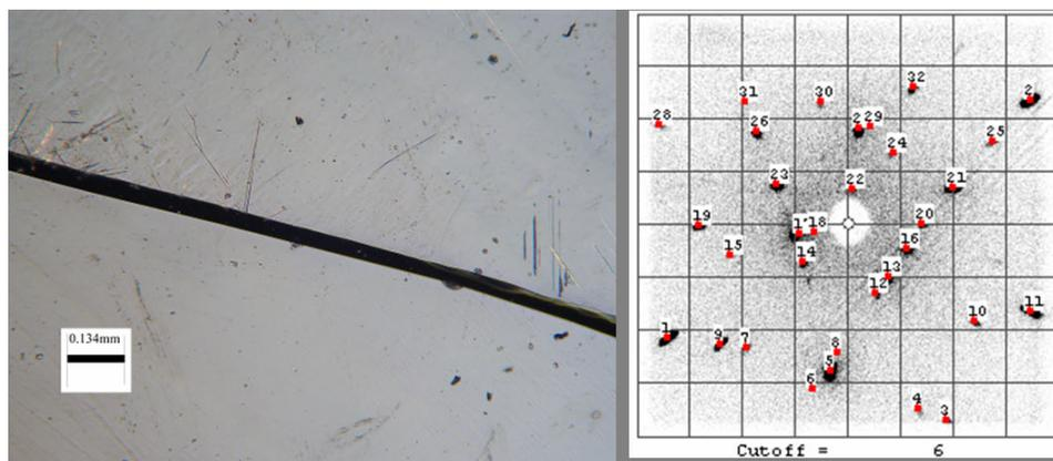
FIG. 2: sample 1 after 900 C heat treatment for 1 hour with known grain boundary, back reflection Laue method pattern taken from above grain boundary
