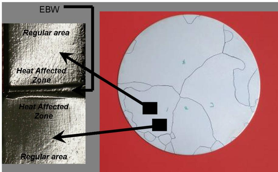
FIG. 8: two pieces of single crystal niobium that were electron beam welded together. These two pieces were extracted from the same parent single crystal niobium
