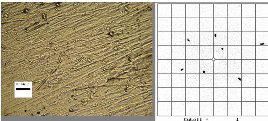
FIG. 7: sample 2 after plastic deformation and 1400 C heat treatment for 2 hours and back reflection Laue method pattern
