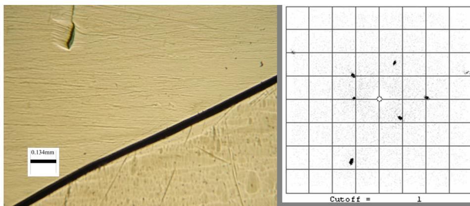
FIG. 3: sample 1 after 1400 C heat treatment for 2 hours with known grain boundary, back reflection Laue method pattern taken from above grain boundary
