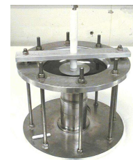
(c) Beam-tube welded half-cell cavity assembly
