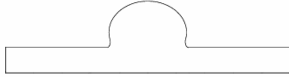
Fig 5: Shape of single-cell cavity.
