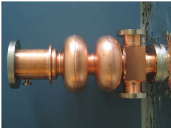
Figure 6: 2-cell injector prototype copper cavity.
