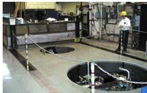
Figure 1: Test pits for various size cavities. Shown is the small and the large pit. Not shown is the medium size pit.
