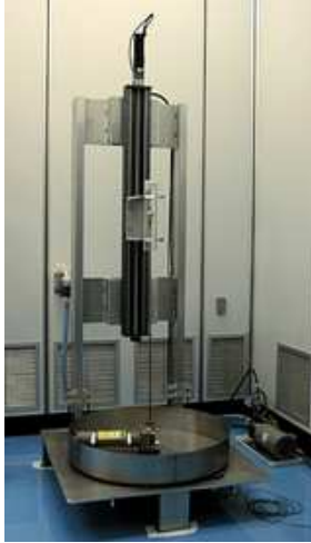
Figure 3: New high-pressure water rinsing system.
